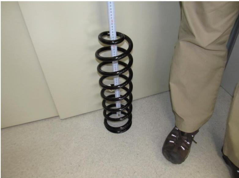
Before fitting measure and note free height of both left and right hand springs.
