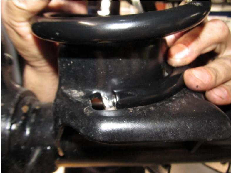
Align spring assembly on bottom seat. There should be approximately 15 mm between the end of the spring and the spring seat.
