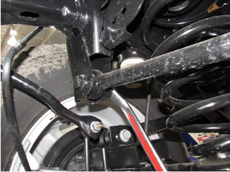
Disconnect the rear panhard rod at the chassis end & back off the torque at axle the end.
