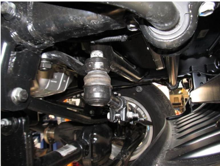
With axle closer to body re connect the drag link and panhard rod.
