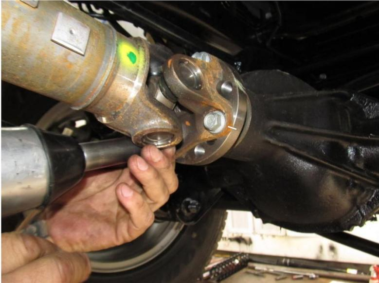
Using a Paint marker, mark driveshaft alignment for re assembly.
