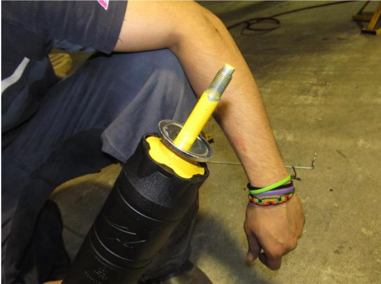
Fit retaining washer and one bushing to the top shock absorber stud.
