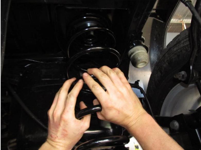
Carefully raise vehicle to remove load on rear springs allowing them to become untrapped.
