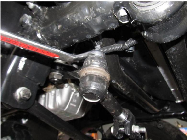
Disconnect steering drag link from the pitman arm. Hold ball joint from spinning with Allen key end of threaded section.
