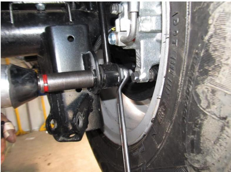
Remove rear sway bar links on both sides of the vehicle.
