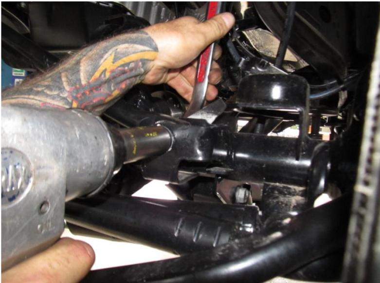
Remove bolt that connects front panhard rod to the axle housing.
