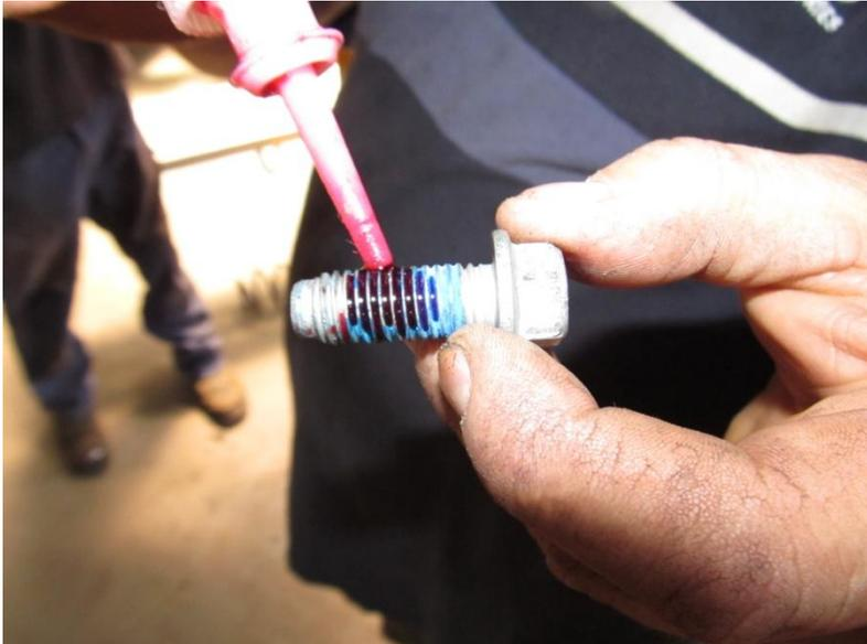
Re apply thread locking compound to all driveshaft flange bolts
