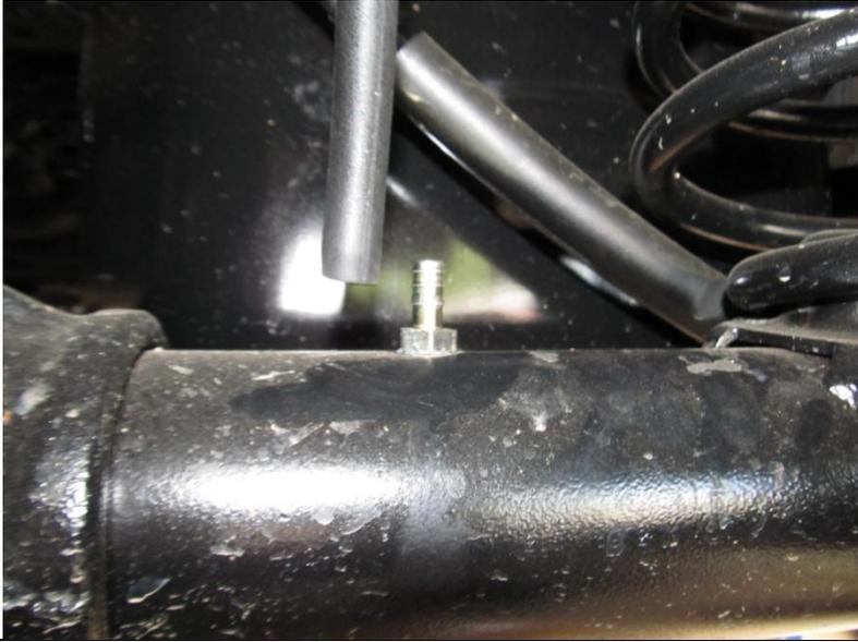
Disconnect rear differential breather tube from axle housing.
