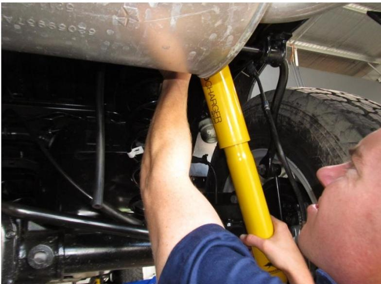
Fit new shock absorber to top mounting position using original bolts.
