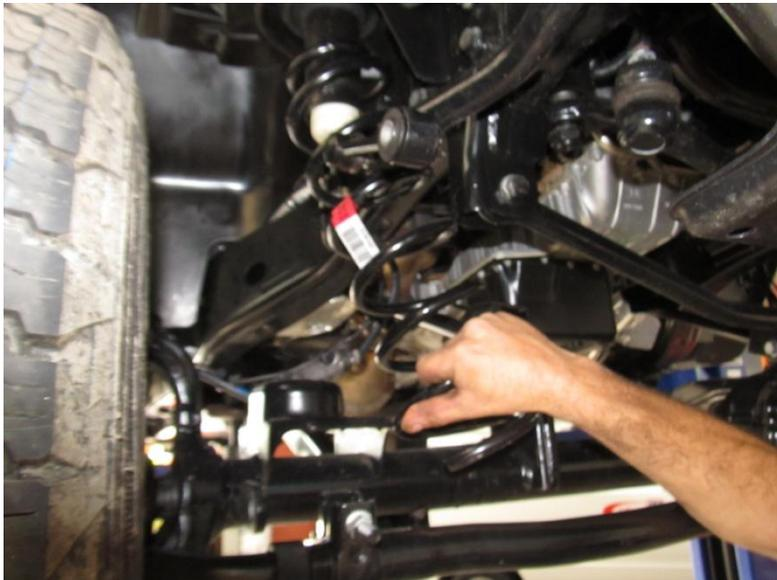
Raise vehicle until springs are no longer captive. Take care to ensure that brake lines and ABS wires are not over stretched.
