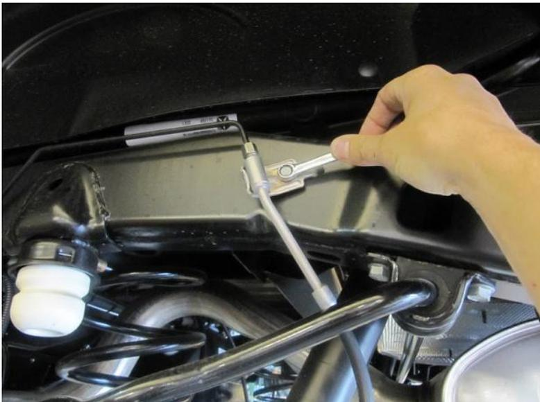
Disconnect the rear brake line brackets on both sides of the vehicle.
