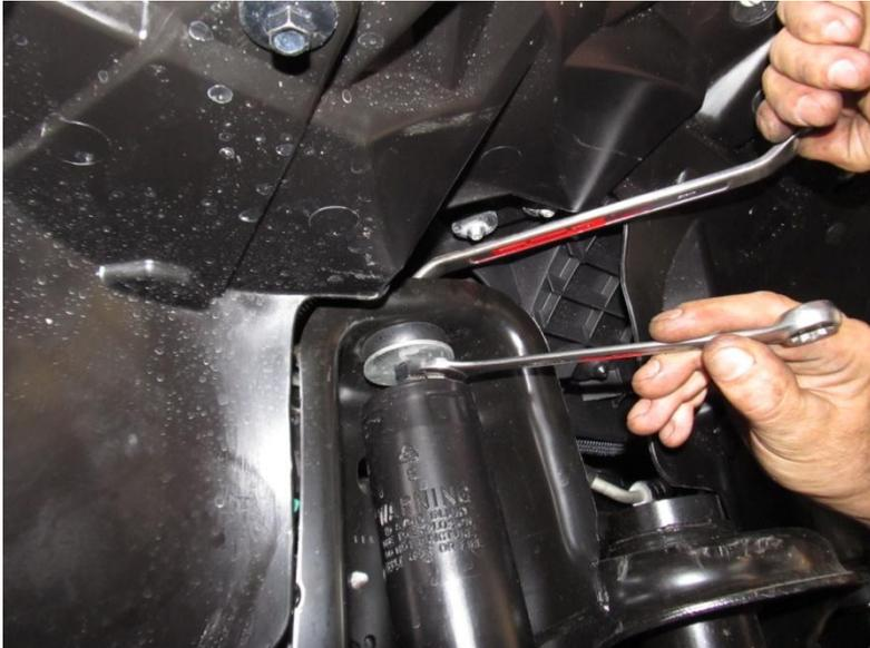
Undo shock absorber top mounting bolt.
