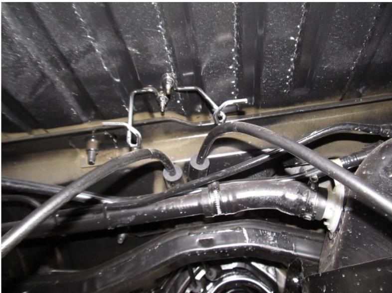
Unclip rear handbrake cable from retaining clip on underside of body.
