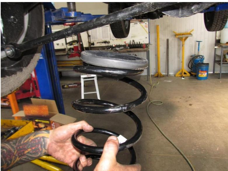
Fit the original rubber spring mounts to the new Old Man Emu springs.
