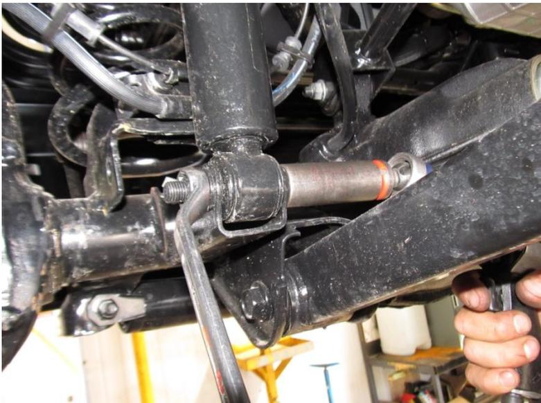
Undo shock absorber bottom mounting bolt.
