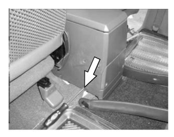
( **B** ) Loosen and remove the original consol mounting bracket. The two mounting points will be used later to secure the Safe to the vehicle.
