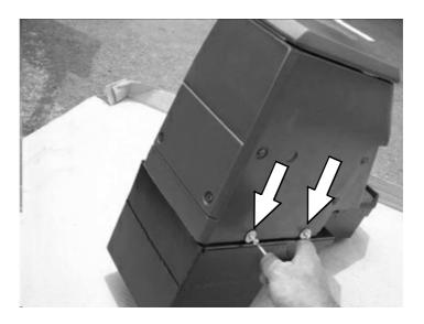
( **F** ) Locate the the front mounting point next to the vehicle's gear lever as indicated by the arrow and place the Aluminium Spacer (Item 6) supplied on top of the mounting point as shown.
