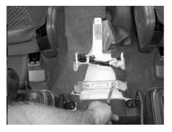
( C ) Loosen and rotate the two seat belt brackets as shown.
