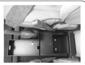
( **H** ) Refit the interior carpet and hidden compartment cover. Close the Safe, remove the key and place the supplied carpet over the lock and front section of the Safe as shown.
