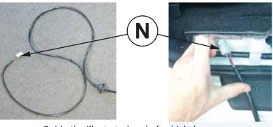
Guide the illustrated end of vehicle loom under the carpet and through the hole that the grommet was removed from in step 3
