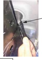
Draw the loom through the hole until the large grommet pops into position
