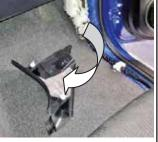
Go to the RH side (driver's) of the vehicle. Open the front driver's door and remove the kick panel by removing plastic nut and prising upwards
