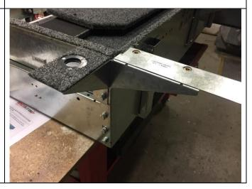
If installing a fridge to the roller floor, it may be necessary to create extra ventilation if the fridges minimum clearances are not met. This can be achieved by cutting the carpet out of the pre-cut holes in the adaptor panel.
