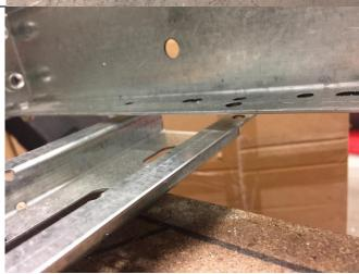
Reinstall M8 bolts to front of drawer. At this time it is recommended to install the desired accessories, eg, barrier impact channels, BEP panels or floor extension brackets.
