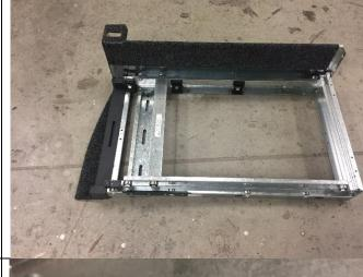
Insert the bottom edge of the adaptor panel between the drawer module and the top hat brackets on the base of the module. Secure the panel to the drawer module by reinstalling the  $4 \times M6$  bolt and nuts to the  $2 \times M6$  top hat brackets.
