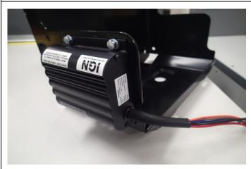
1. Install BCDC to the side of the Battery Tray as shown using M6 x 16 bolts, Flange nuts and Flat washers. Place a washer under bolt head. Tighten to specified torque.
