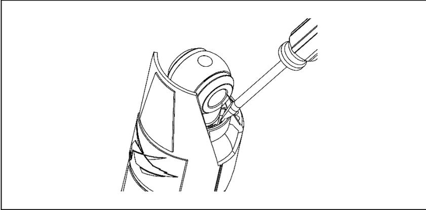
4. Check Retainers are completely secured by Guard. Use a flat blade screwdriver to poke Retainer under tab on guard if required.
