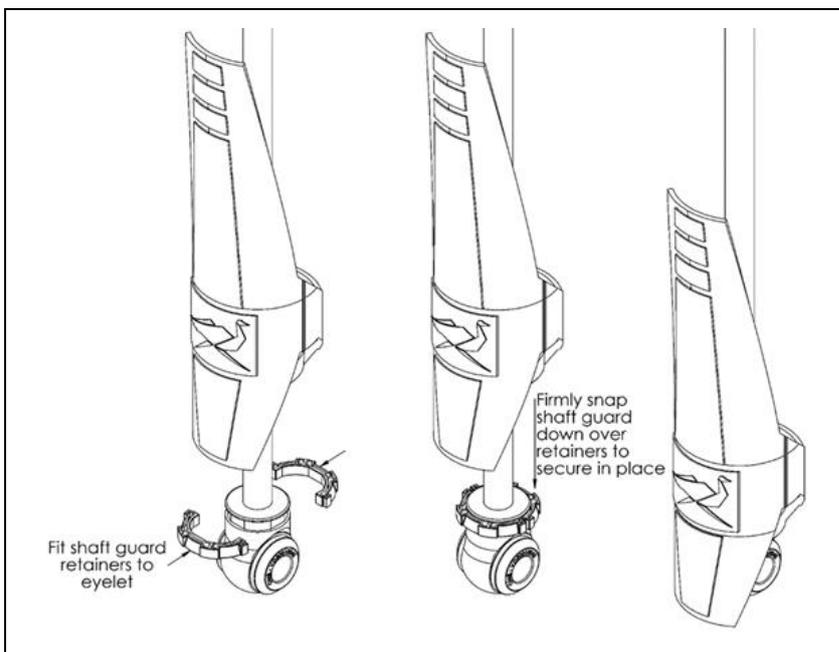
Guards can be mounted to the Eyelet with Damper Bolt mounted from the side or from the front.
