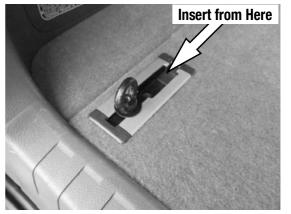
(C) Secure the front and rear of the Drawer System to the vehicle using the Turnbuckles and C-Hooks (Items 2, 6, 8, 10) as shown below. Ensure the Drawer System remains in position while tightening the Turnbuckles.
