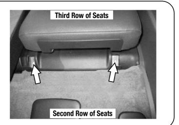
(**B**) Secure the left and right hand Mounting Brackets (Item 14) to the vehicle as shown below, using the original bolts removed in Step 2A.
