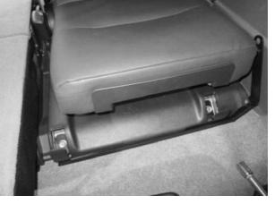
(**C**) Loosen the round end of the two Turn Buckles (Item 2) supplied with SSDR005 and assemble a M6 Wing Nut (Item 3) as shown. Reassemble the Turn Buckle.
