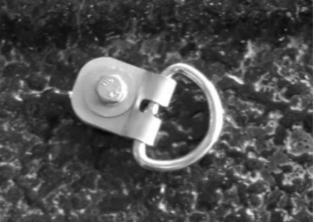
(**I**) Remove the four tie down hooks from the vehicle's loadbay.
