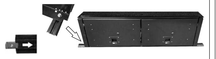
(E) Looking at the rear of the Drawer System, remove the bolts as indicated by the arrows. Keep the bolts and washers safe as they will be used at a later stage.
