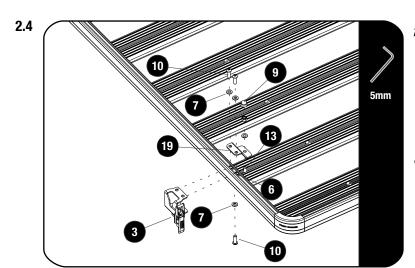
Place the Rack Mount Brackets (Item 2) over the other the side profile, followed be the Rack Support and secure using M8 x 25 Button Head Bolts, M8 x 16 Hex Bolts, M8 x 16 x 1.6SS Flat Washers and M8 Nyloc Nuts (Items 5, 6, 7, 10 & 13) as shown.
