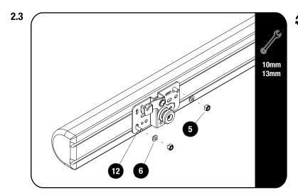
Loosely fit the assembly from 2.2 onto the back of your awning. Depending on the make of your awning use either M6 x 16 or M8 x 16 Hex Bolts, Nyloc Nut and Flat Washers. (Items 12, 16 & 17 or 5, 7 & 13) as shown.
