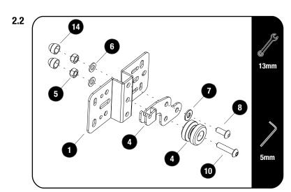
Assemble the Bobbins and Catches (Items 3 & 4) to the Awning Mount Brackets (Item 1) using a M8 x 20 Button Head Bolts, M8 x 35 Button Head Bolts, M8 x 19 x 2SS Flat Washers, M8 x 16 x 1.6SS Flat Washers and M8 Nyloc Nuts (Items 5, 6, 7, 8 & 10) as shown.
