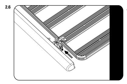
Place the loop of the latch over the hook of the Catch on the Mounting Bracket.
