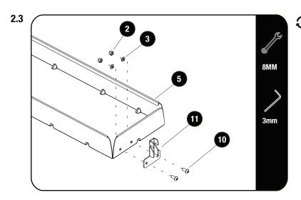
Secure the Latch Keeper (Item 11) to the Jerry Can Holder Base (Item 5) using two M5 x 12 Button Heads, two M5 Flat Washers and Two M5 Nyloc Nuts (Items 10, 3 & 2) as shown.
