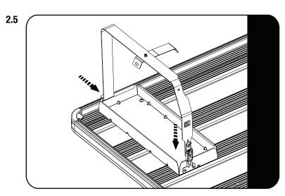
Insert the Top Strap into the slot in the Jerry Can Holder Base.
