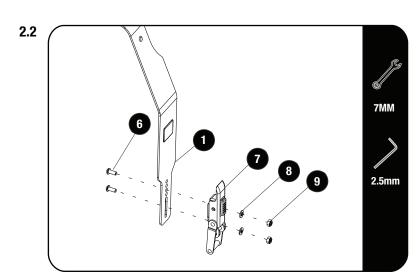
Loosely fit the Latch (Item 7) to the Top Strap (Item 1) using M4 x 10 Button head, M4 Flat Washers and M4 Nyloc Nuts (Items 6, 8 & 9) as shown.
