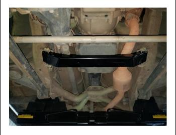
2. Fit ARB crossmember using original fasteners.
