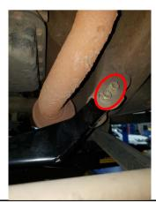
Torque fasteners to specification (LHS shown).
