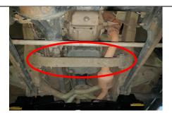
Remove 4x fasteners from crossmember. Remove crossmember from chassis, retain fasteners (LHS shown).
