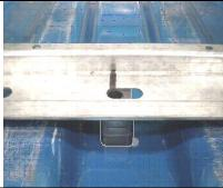
**2.14/-** Bolt frame down through drilled holes using four (4) M10x60mm bolts, M10x70x40 flat plates inside the vehicle and weatherproof plates and Nyloc nuts on underside of vehicle.
