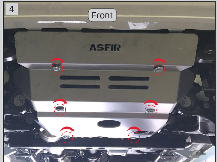
Connect plate (A) to the original screwing using 6 hex bolts (B) with spring washer (c) and pocket washer (D). Tighten the bolts
