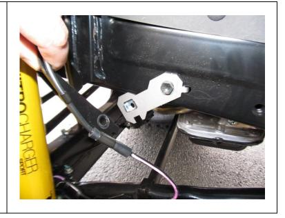
3. Fit factory ABS wire bracket to relocation bracket as shown and secure with M8 x 16 bolt, spring washer and flat washer supplied.
