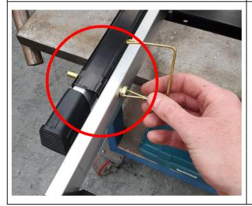
1.6) Locate 8mm wire lock pin (6152216) through hole.
