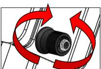
3.0) To use the extension ladder levelling legs, loosen cam handle on side of ladder. Extended the desired amount, lock the extension legs with the compression cam handle. Adjust the locking nut to increase or to decrease the locking force if required. Ensure they are securely locked.
