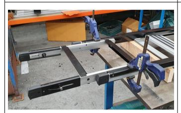
1.2) With extension ladder brackets in place use G-clamps to hold extension ladder in the centre of the bracket tightly in place against the extension legs of the RTT.
