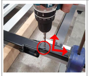
1.7) Locate top face hole in U bracket on the outside RH side of the ladder. Drill an 8mm hole through this hole keeping perpendicular to surface.
