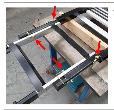
1.10) With four wire lock pins in place and the wire loops locked over the ends of the pins, the ladder extension accessory is now fully fitted to the ladder for the tent
