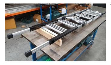
1.0) Place the ladder from the Altitude tent (RTT) horizontally on flat surface with step tread surface facing up. Place a cross-wise chock about 10cm in height, under bottom end to elevate legs of the ladder into free space.
