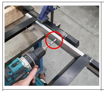
1.4) Now locate 8mm dill bit to corresponding inside hole pre-drilled on the extension ladder (561AS003). Drill through one surface only of the RTT extension leg extrusion. The hole inside needs to align to the outside hole drilled in the previous step of these instructions.
