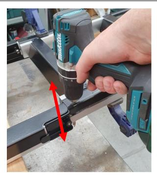
1.8) Once both holes are drilled right through RTT ladder extension leg, pass the drill bit back and forward through 8mm hole to make sure the 8mm wire lock pin (6152216) can pass through and be fitted.
