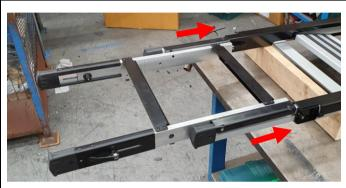
1.1) Straddle the ladder extension accessory (561AS003) with the U - shaped side brackets over each of the RTT ladder extension legs. Push the ladder extensions (561AS003) up the tent ladder until the U brackets fit flush with bottom extrusion of the RTT ladder.
