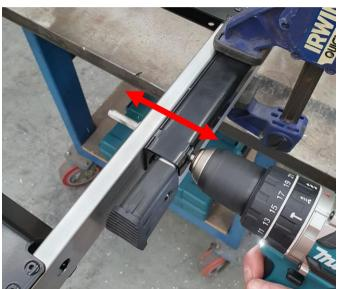
1.5) Once both holes are drilled through RTT extension leg pass the drill bit back and forward through 8mm hole to make sure the 8mm wire lock pin (6152216) can pass through.
