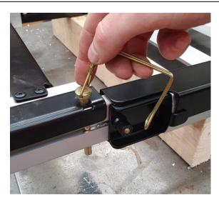
1.9) Install the 8mm wire lock pin (6152216) through U bracket and drilled hole.
