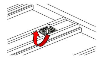
1.4 Rotate the stud plates on the BASE RACK 90 degrees and remove from the base rack channels. Discard the coach bolts (20mm) in the stud plates.
