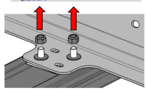
1.3 Unscrew the M8 Nyloc nuts securing BASE RACK to the blade brackets and carefully remove the blade brackets.
