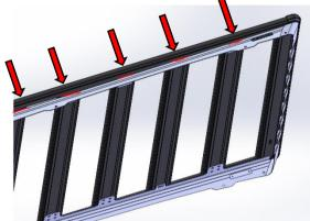
1.2 Flip the BASE RACK assembly upside down and mark the location of the Blade Brackets on the BASE RACK.
