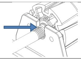
Tighten both knobs a further three and a half turns after initial contact of the knob to the clamp. Align the nearest hole in the knob with either hole on the clamp. Insert the detent pin through the aligned hole on the knob and clamp. Rotate the knob slightly again against the detent pin.
