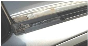
10.Remove the exterior roof trim from both sides of the vehicle. Take care not to bend the trim, as it will be reused.
