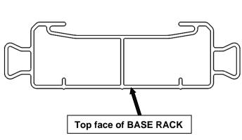
24. Place the BASE RACK face down on a clean flat surface. Provide protection to the top face of BASE RACK to avoid marking of surfaces
