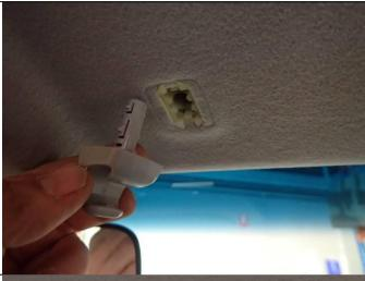
2. Remove the plugs located around the periphery of the ceiling. They are located at the front at the driver's side, the rear of the ceiling at the right & left side of the vehicle and above the rear windscreen.
