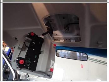
4. Carefully remove centre roof console and unplug.
