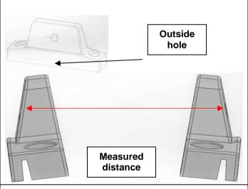
23. Using a tape measure, measure across the vehicle between the middle of the hole on the outside face of the front and rear set of mounting brackets. Make a note of each measurement.
