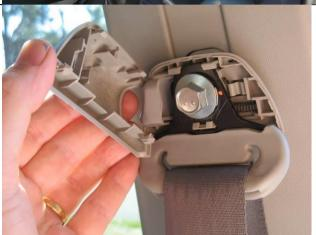
6. Remove the front and rear top seatbelt mounts. Do not use power tools to remove or install seatbelt hardware.
