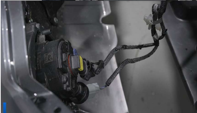
13. Disconnect wiring from the lights
