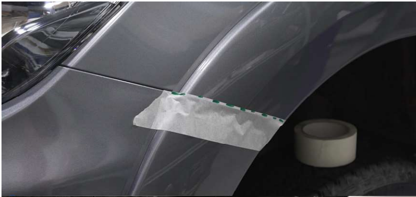
10. Mark the pad cutting line
