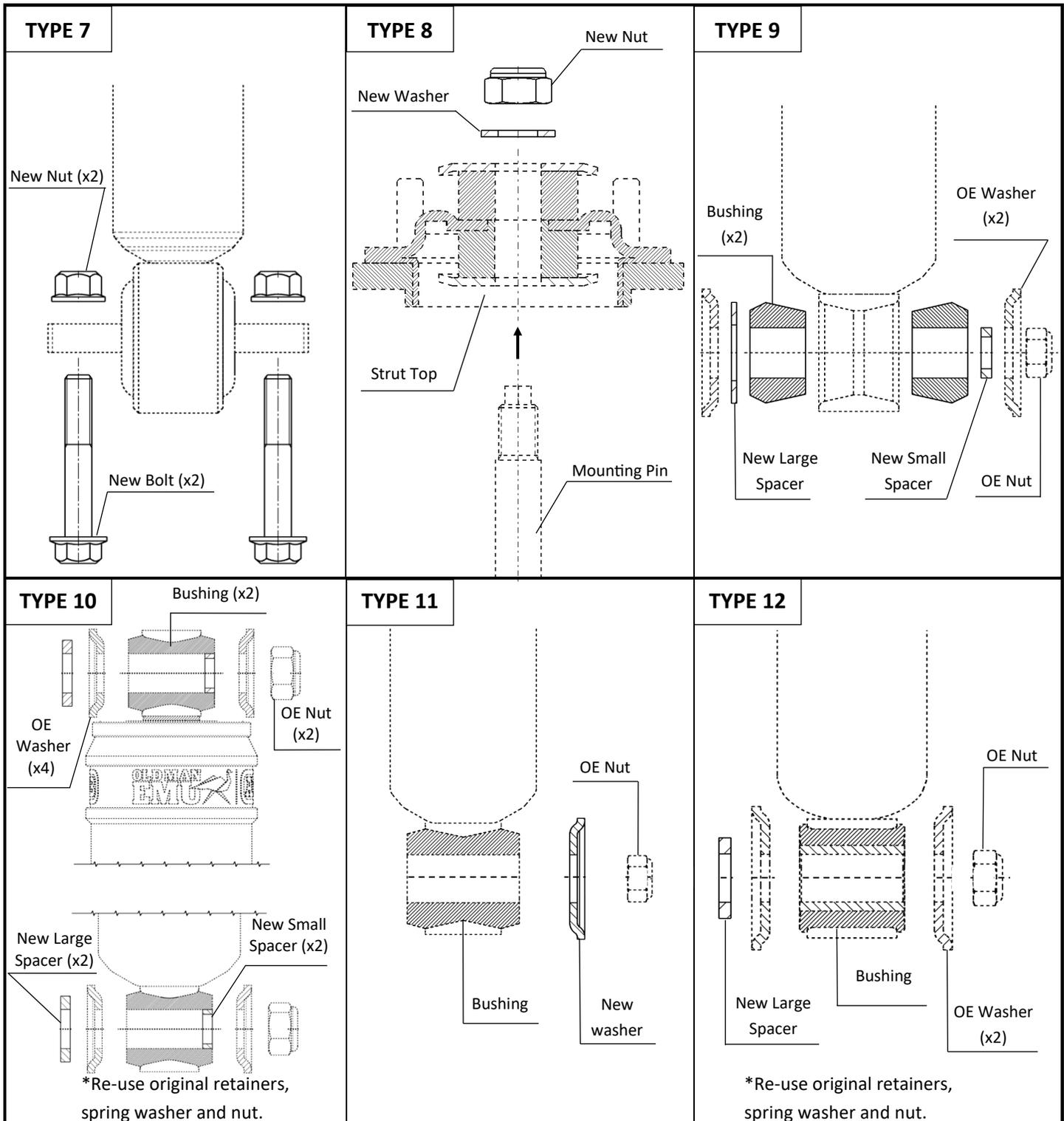
• To ensure correct fitment of small mounting parts reference type number on SMP bag to above chart
